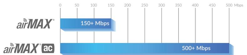
\* Up to 330+ Mbps (maximum 40 MHz channel width) for PtMP links.
